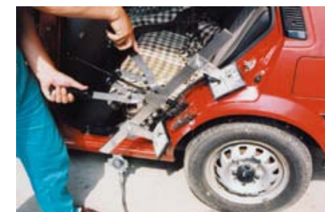
Pulling and hammering
