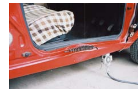
Weld the bits on the line
