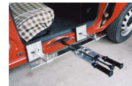
Lock the handles and planish under tension
