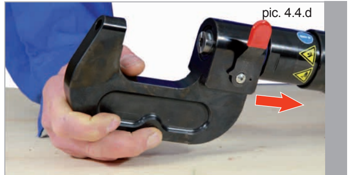
4. Push the C-arm onto the intake of the short stroke cylinder.
