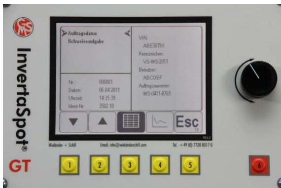
Button 3 will open the graphic display
